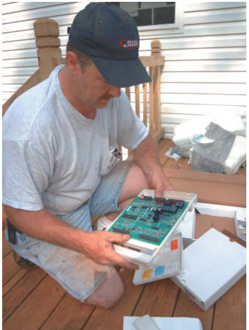
Figure 5. The “user interface” circuit board is the brain of the comfort system; it continually adjusts the air handler, outdoor heat pump, and zone dampers based on sensor input and its programmed instructions. The board shown, a Bryant Evolution control, is capable of managing a wide variety of mechanical systems and can serve as many as eight independent zones.
