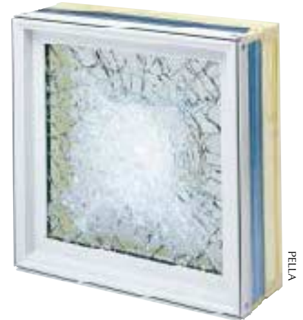
Figure 1. To keep hurricane-force winds out of the house, impact-resistant windows have to sustain a 34-mph hit from an airborne 2x4. They can crack, as shown, but not shatter.
