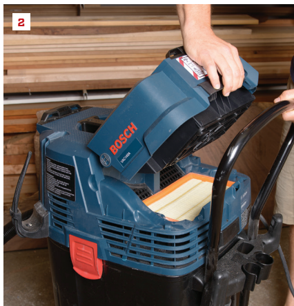
2. Simply lift a hinged lid to access the filter. 3. The vacuum sucked up 25-pound bags of drywall compound in an average of 80 seconds per bag.
