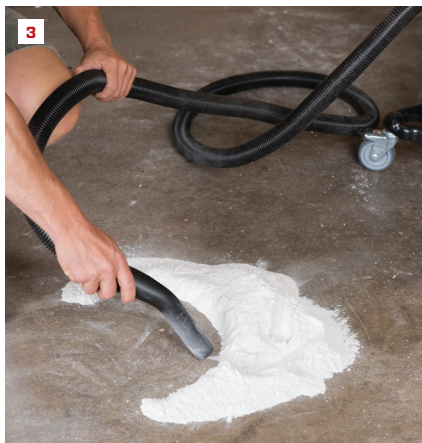
2. Simply lift a hinged lid to access the filter. 3. The vacuum sucked up 25-pound bags of drywall compound in an average of 80 seconds per bag.
