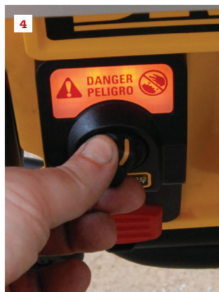
1. The maximum rip capacity is a class-leading 32 1/2 inches to the right of the blade. 2. A low auxiliary fence flips down next to the main rip fence to make narrow ripping safer and easier. 3. To install the blade-guard assembly, simply pull the external release lever and slip the guard into position. 4. The DWE7499GD adds a unique Guard Detect on/off paddle switch that warns you with a flashing light when the blade guard isn't properly installed. To work without the guard, you must turn the bypass knob each time you turn on the saw.
