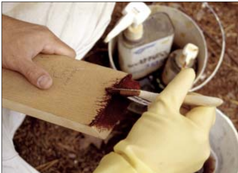
Sealing end grain with a marine-grade epoxy prevents the wood from soaking up water.
