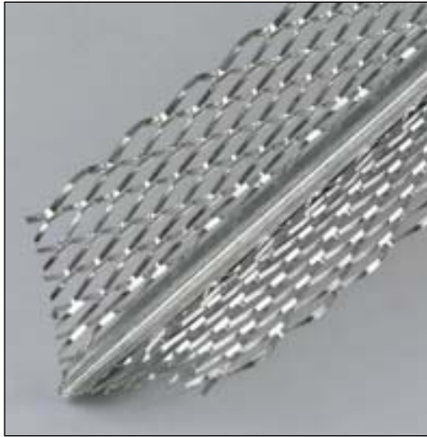
FIGURE 1. CORNER BEAD. To prevent stucco from popping off at outside corners, use corner bead. An alternative (not shown) is to round the corner, allowing the lath to poach out and provide plenty of room for stucco to key to the lath. The end result is a rounded corner that may not be compatible with all architectural styles.
