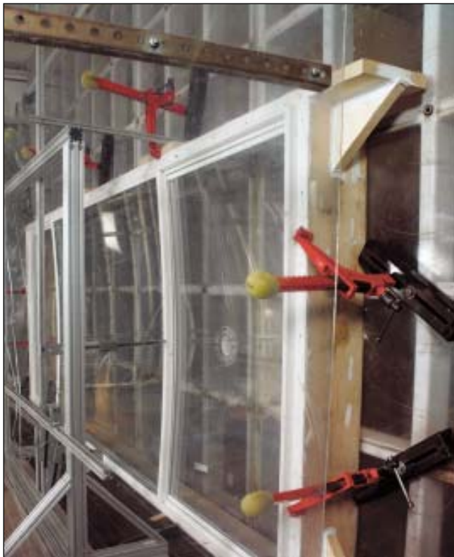
FIGURE 5. The Pressure Test: In the laboratory, wind pressures applied to a window in a high-wind event are simulated by applying a static pressure across a random window specimen for a prescribed amount of time and measuring the maximum uniform load deflection.
