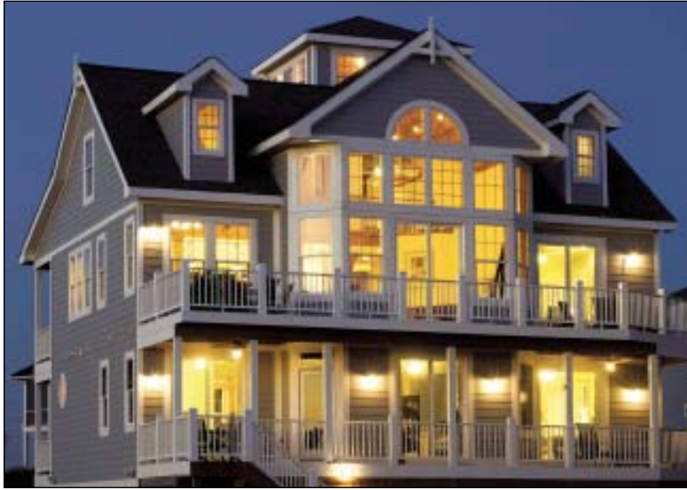
FIGURE 2. Just a couple years ago, windows featuring impact-resistant glass were available in only a limited range of sizes. Now manufacturers competing in the coastal market offer a range of windows with a wide range of design pressures, making compliance with the International Residential Code wind requirements much easier.
