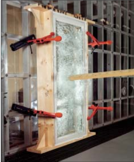
FIGURE 3. An impact-resistant window can shatter and still pass the large missile test if the window remains largely intact through the 9,000 pressure cycles. The glass fragments tend to adhere to the plastic interlayer, which is considered intact if the size of any rips that develop during the test total less than \frac{1}{16} inch wide by 5 inches long.
