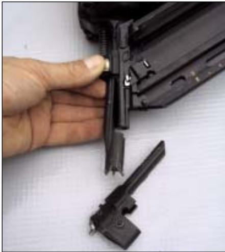
FIGURE 6. The Bostitch F 33 — a full-size framing nailer — converts to a metal connector nailer by switching out the nosepiece. This is the only metal connector nailer that can handle the 3-inch-long nails required for the “double-shear” or diagonal location required in some hangers.
