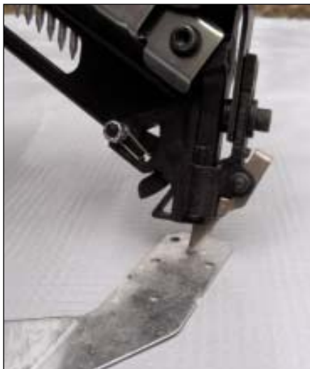
FIGURE 4. Paslode (left) and Max (above) use a safety probe that both indexes the hole and prevents the tool from firing if it’s not in a hole. This probe pivots out of the way when the nail fires.
