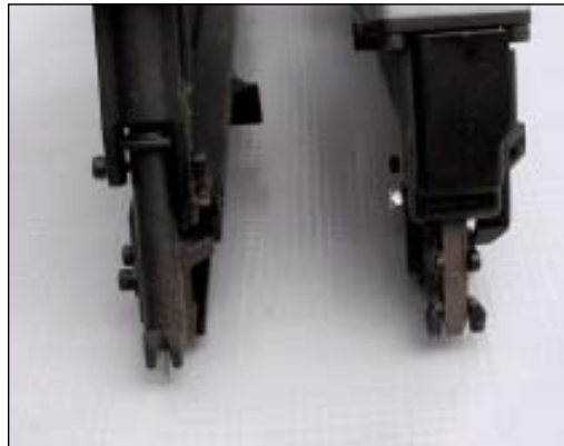
FIGURE 3. To prevent ricochets off the metal connector, manufacturers rely on a variety of different nose designs. The Bostitch StrapShot tool (left photo) has a streamlined barrel that moves the thickness of a metal connector. The gun won't fire unless the nail is in the hole, and the geometry of this barrel prevents the tool from firing at a steep angle. PneuTools relies on the travel of the whole front end, not just the nosepiece, but includes a forked yoke that will prevent a misfire at a steep angle (right photo, left image). Hitachi relies on both: a wide yoke prevents angled misfires and a sensing finger that can "feel" the nail in the hole will prevent firing outside of the hole (right photo, right image).
