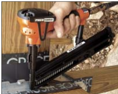
FIGURE 1. The big advantages of multi-blow hammers are safety and control: there's no chance of a ricochet off the hardware, and it's easy to seat the nail properly.
