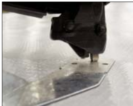
FIGURE 4. Paslode (left) and Max (above) use a safety probe that both indexes the hole and prevents the tool from firing if it’s not in a hole. This probe pivots out of the way when the nail fires.
