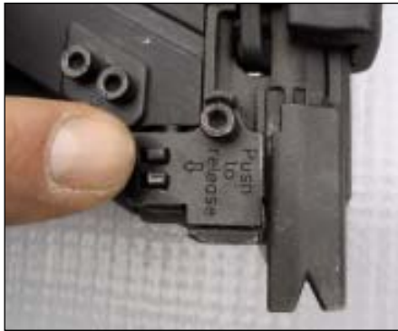
FIGURE 5. A tool that uses the nail to index the holes can potentially jam if the tool is pressed forward while the nail is in the hole. This causes the collation to back out slightly, so the nail is misaligned with the driver blade. Only the Bostitch StrapShot (left) prevented this with a pawl that slips down between nails and prevents the collation strip from backing out.
