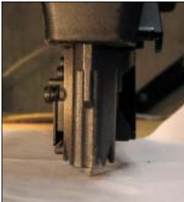
FIGURE 3. To prevent ricochets off the metal connector, manufacturers rely on a variety of different nose designs. The Bostitch StrapShot tool (left photo) has a streamlined barrel that moves the thickness of a metal connector. The gun won't fire unless the nail is in the hole, and the geometry of this barrel prevents the tool from firing at a steep angle. PneuTools relies on the travel of the whole front end, not just the nosepiece, but includes a forked yoke that will prevent a misfire at a steep angle (right photo, left image). Hitachi relies on both: a wide yoke prevents angled misfires and a sensing finger that can "feel" the nail in the hole will prevent firing outside of the hole (right photo, right image).
