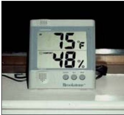
FIGURE 4. Prices for a digital hygrometer range from about $30 to $300, but a low-cost model such as this one is sufficient for most remodelers. This tool is primarily an aid for talking to clients about temperature and humidity and explaining the causes of condensation on glass even when it's not visible.
