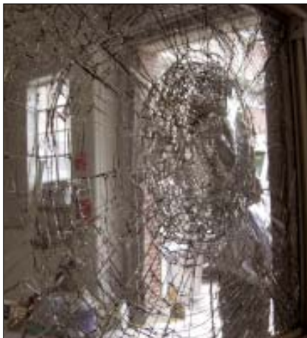
FIGURE 1. Windows that meet the ASTM E 1886 and ASTM E 1996 impact standards shatter but do not present an opening that will either pressurize the interior or allow undue amounts of water into the home (above). However, most conventional wall systems do not fare as well under the same test. A typical vinyl-sided wood-frame wall is obliterated by the large missile test (right). A concrete block wall performs a bit better but still allows a sizable hole for wind and water to penetrate (top right).
