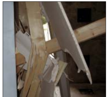
FIGURE 1. Windows that meet the ASTM E 1886 and ASTM E 1996 impact standards shatter but do not present an opening that will either pressurize the interior or allow undue amounts of water into the home (above). However, most conventional wall systems do not fare as well under the same test. A typical vinyl-sided wood-frame wall is obliterated by the large missile test (right). A concrete block wall performs a bit better but still allows a sizable hole for wind and water to penetrate (top right).
