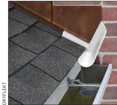
FIGURE 7. Details to keep rainwater from flowing behind the brick are the first line of defense. Above, a DryFlekt polypropylene kickout diverter flashing has been integrated into copper step flashing to direct water into gutters rather than letting it soak into the brick wall.
