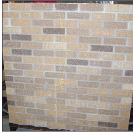
FIGURE 2. In standard impact testing at Texas Tech University, a 9-pound 2x4 launched at 35 miles per hour punctured a wood wall section sided with fiber-cement (above left), but bounced off brick veneer, leaving barely a scratch (above right).
