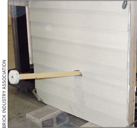
FIGURE 2. In standard impact testing at Texas Tech University, a 9-pound 2x4 launched at 35 miles per hour punctured a wood wall section sided with fiber-cement (above left), but bounced off brick veneer, leaving barely a scratch (above right).
