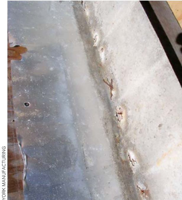
Figure 1. Aluminum has been the go-to flashing for decades, but contact with ACQ and CA preservatives corrodes the metal. And some studies have shown aluminum to corrode too quickly near the coast, even with the less corrosive CCA preservatives of the past.
