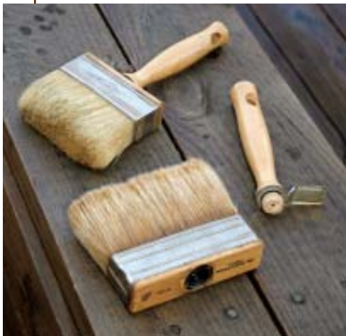
Figure 12. The slowest way is best. Most finishes can be sprayed, but the author gets the best results from China bristle brushes. For speed and a healthy back, get brushes with handles that can be removed and replaced with a broomstick.
