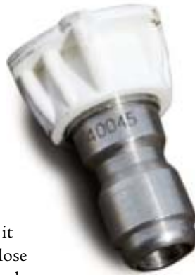
Figure 9. Use the right tip. The first two numbers on a pressure washer tip indicate the width of the spray fan. This one is 40 degrees, right for washing decks. The next three numbers are the flow, in this case 4.5 gpm. To avoid damaging the machine, always use tips with a greater flow capacity than the machine can provide.
