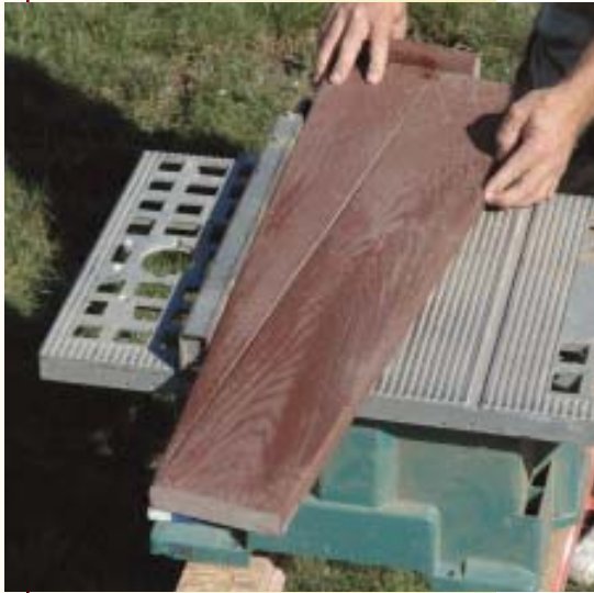
Figure 10. Straight-edged wedges require a jig. This is the sort of work where errors accumulate, so accuracy is called for from the start.
