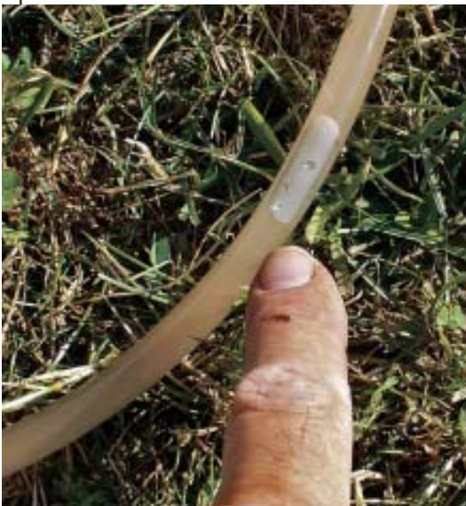
Figure 5. Bubbles in the fluid ruin a level's accuracy. To get rid of them, simply refill the tube. Kinks are bad, too, so don't step on the hose. Finally, a temperature differential can affect accuracy, so avoid using a water level half in the sun and half in the shade.
