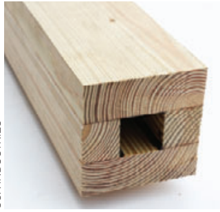
Figure 2. Laminated deck columns are less likely to twist or bow than solid timbers, and the hollow type allows for hidden wiring of lamps.
