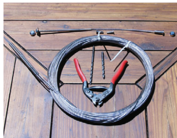
Figure 4. The system used by the author comes with the threaded adjuster already attached to one end of the cable.
