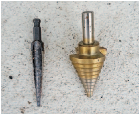
Figure 8. Step drills work great on steel and allow one bit to drill holes of several sizes.
