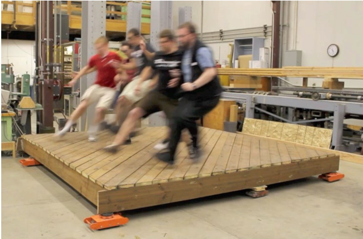
Figure 1. Impulse Loading Caused by Occupants Leaping/Stopping in Unison
