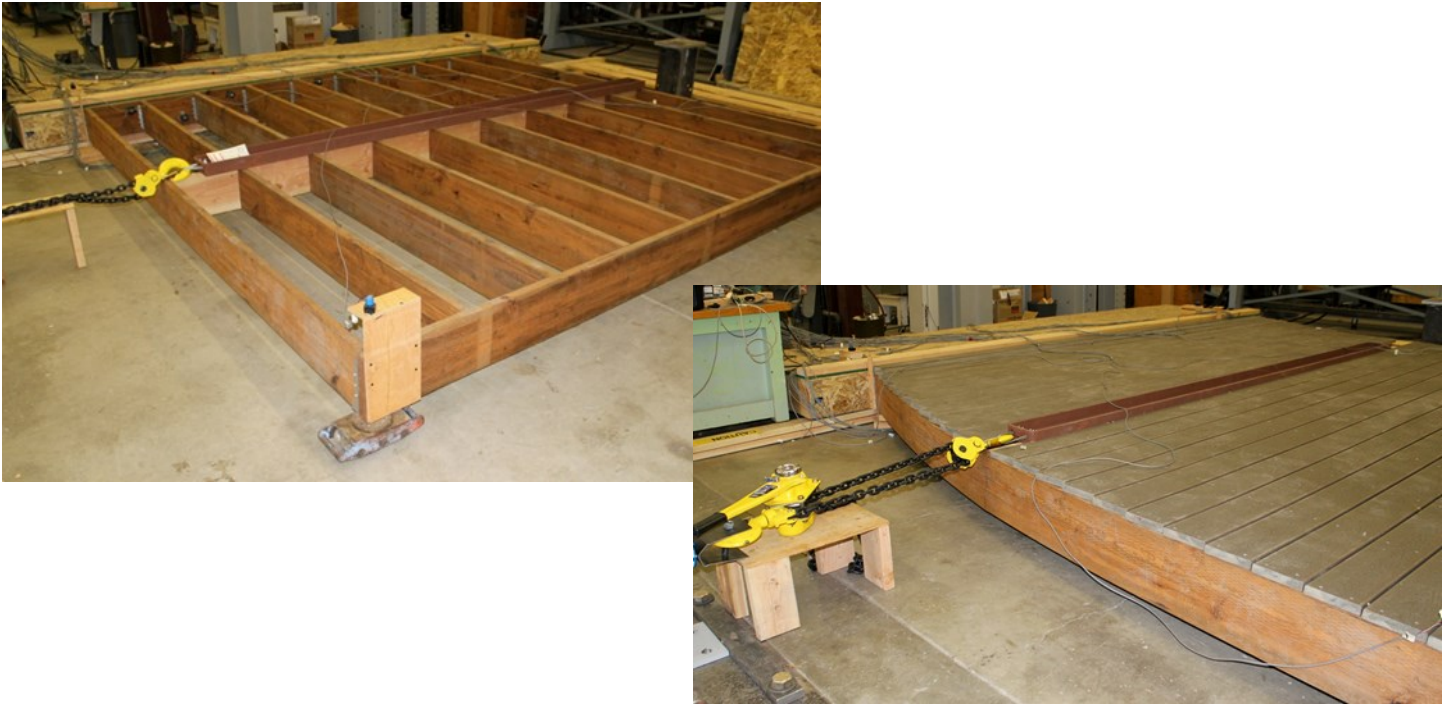
Figure 2. Load Application Setup Showing Framing and Blocking
