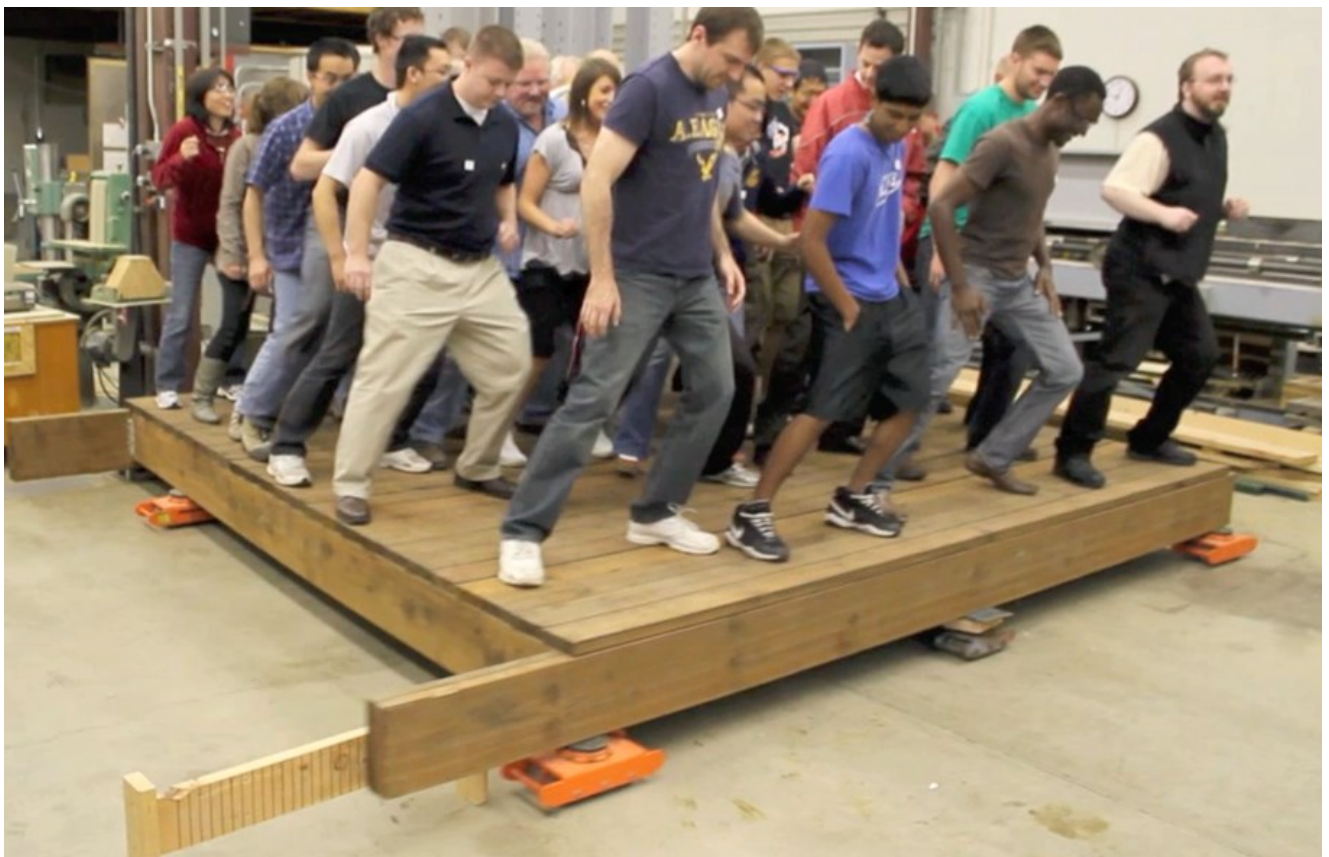
Figure 2. Cyclic Loading Caused by Occupants Swaying Side to Side in Unison
