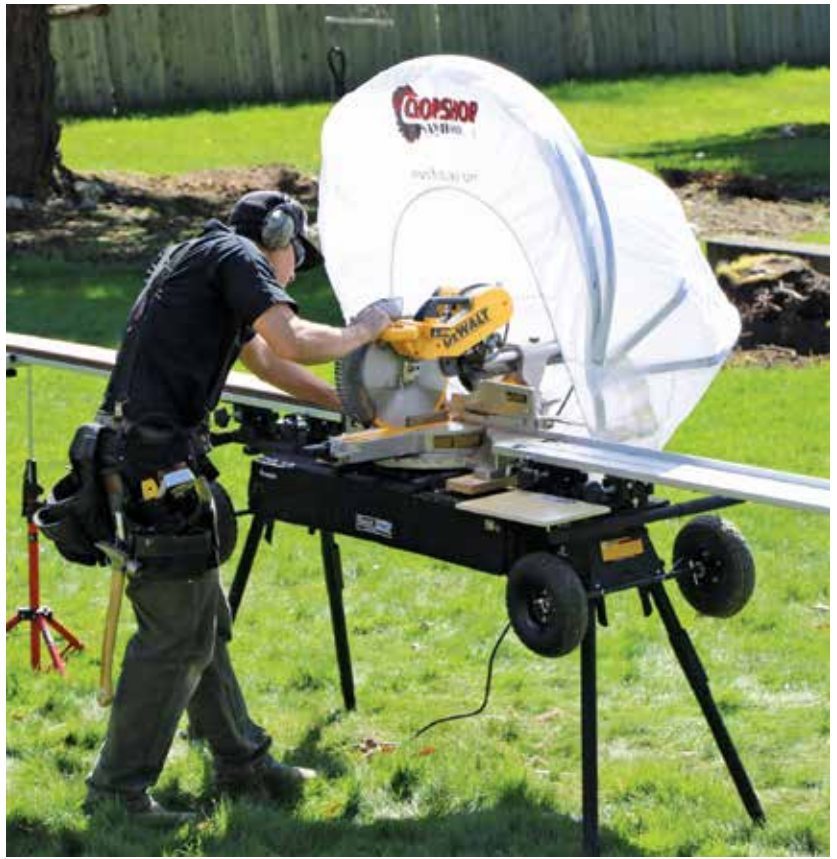
Figure 3. The optional chop-saw hood contains dust and can be used to help keep the saw dry in wet weather.
