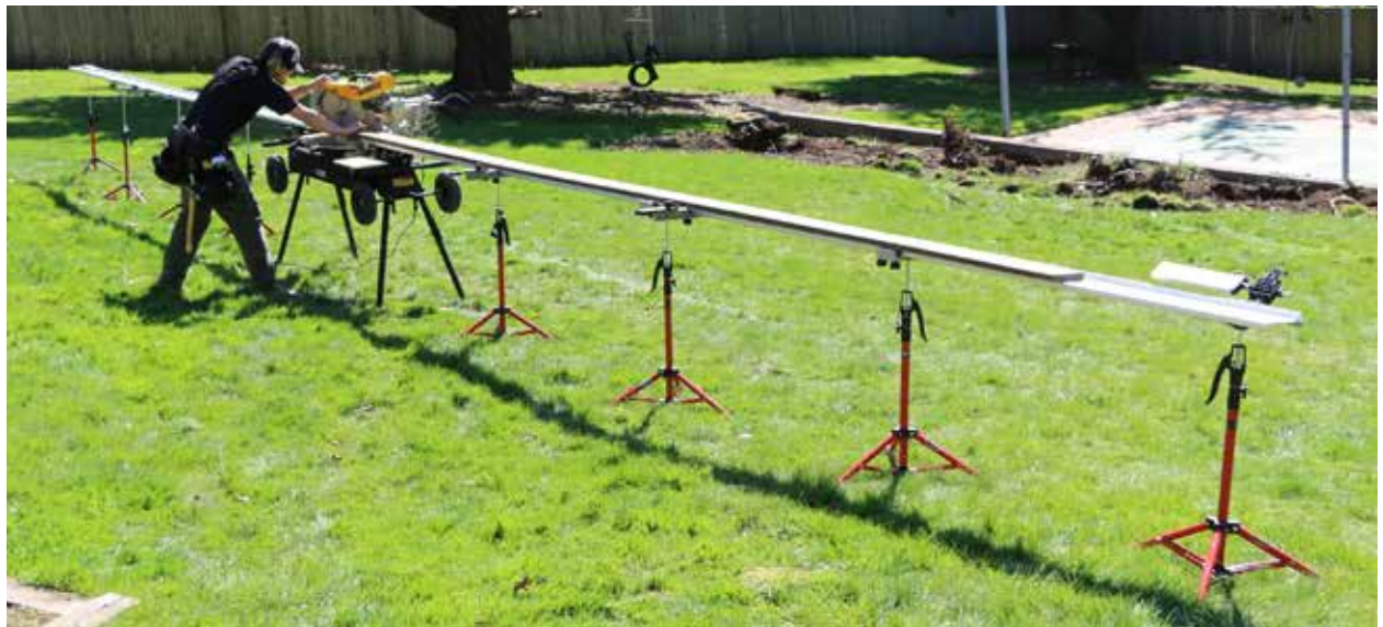
Figure 1. The saw stand has integral wheels that allow it to be easily moved over rough terrain, and it can be customized with additional fence sections and supports to fit long decking stock.
