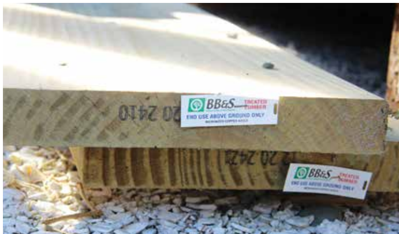
Figure 3. Each stick of treated lumber has a label that identifies the chemical formulation that it has been treated with. Retention levels for different formulas and different uses are established by the AWPA or by code evaluation reports, such as ICC-ES reports.
