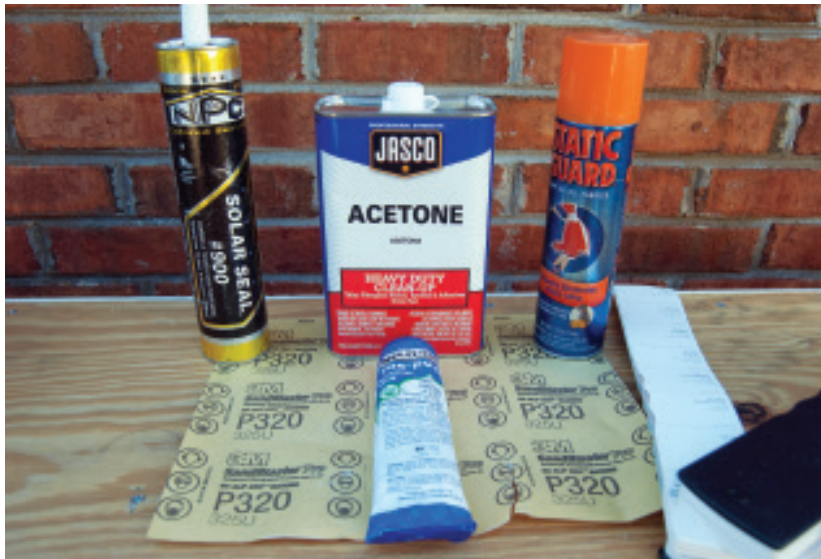
Figure 7. When you're working with cellular PVC, the right adhesives and sealants and a few specialty items will result in a better-looking job.
