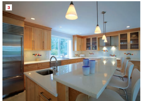
Recessed downlights are a common option for ambient kitchen lighting (1) . A flush-mount light in the center of the kitchen can work in concert with pendants over a peninsula (2) , or pendants above an island can provide ambient light on their own (3) .
