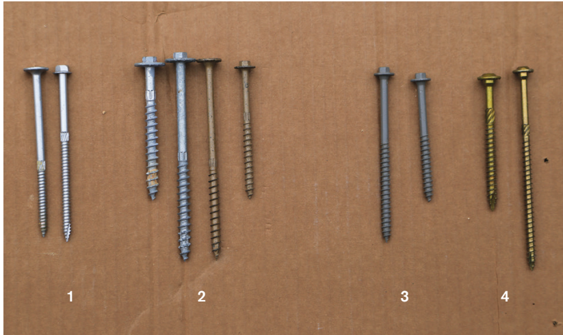
Figure 7. Proprietary structural screws don't require predrilled holes and have a wider positioning range through the ledger, rim joist, and even the mudsill or wall plate. Pictured (from left to right): 1. Mitek WSW Pro Series washer head and hex head exterior screws; 2. Simpson Strong-Tie SDWH HDG (short and long) screws, coated SDWS, and coated SDWH Timber-Hex screws; 3. FastenMaster LedgerLok (long and short) screws; 4. GRK RSS (short and long) screws
