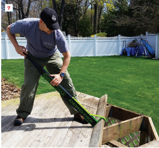
The Demo-Dek (7) has a beefy laminated bamboo handle and an alloy steel jaw design that allows the tool to remove deck boards without relying on a joist or a beam for leverage.
