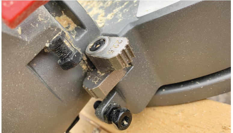
Precise cuts are easy, thanks to the visibility offered by the louvered blade guard (left) and fine-tuneable 22.5-degree and 33.9-degree bevel detents (above).
