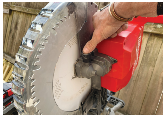
The blade guard rolls up and out of the way for access to the arbor during blade changes (top). There's a push-button spindle lock on the right-hand side of the blade (above).
