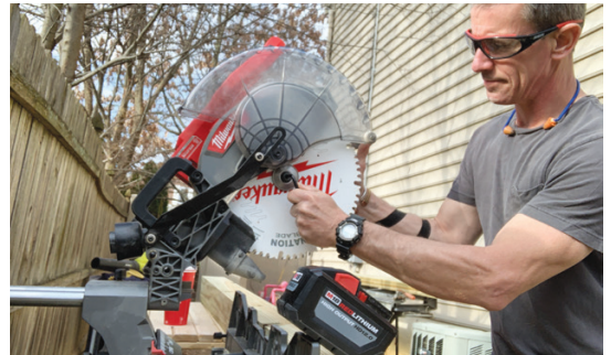
Precise cuts are easy, thanks to the visibility offered by the louvered blade guard (left) and fine-tuneable 22.5-degree and 33.9-degree bevel detents (above).
