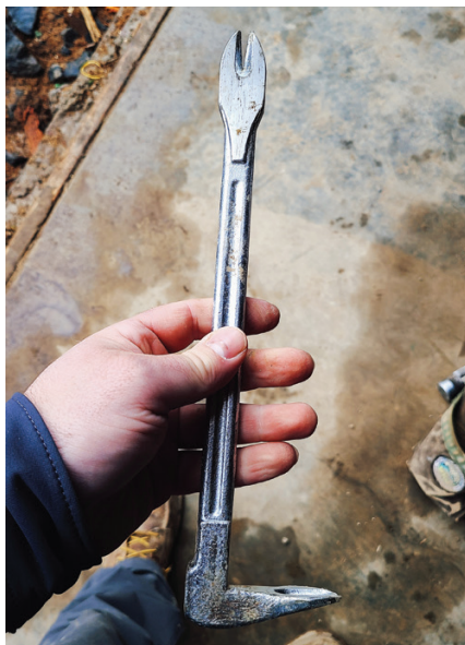
The Dalluge Da Bar is a tough nail puller with flat claws that can slip easily under trim without damaging it.
