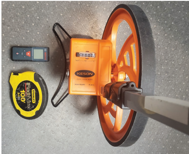
The author's tools: laser measure, measuring wheel, and long tape measure.
