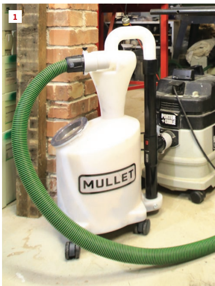
The parabolic cyclone that forms the top section of the Mullet M5 Cyclone Dust Collector scrubs dust particles out of the air before they fill up the vacuum cleaner bag or clog up the filters (1). A simple thumbscrew connects and disconnects the Mullet from the vac with ease (2). Every time the 5-gallon-capacity dump bin fills up, a dust bag lives to fight another day (3).
