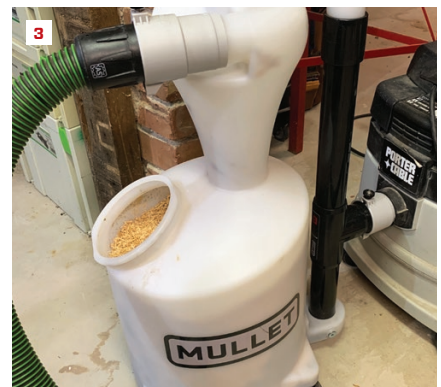
The parabolic cyclone that forms the top section of the Mullet M5 Cyclone Dust Collector scrubs dust particles out of the air before they fill up the vacuum cleaner bag or clog up the filters (1). A simple thumbscrew connects and disconnects the Mullet from the vac with ease (2). Every time the 5-gallon-capacity dump bin fills up, a dust bag lives to fight another day (3).
