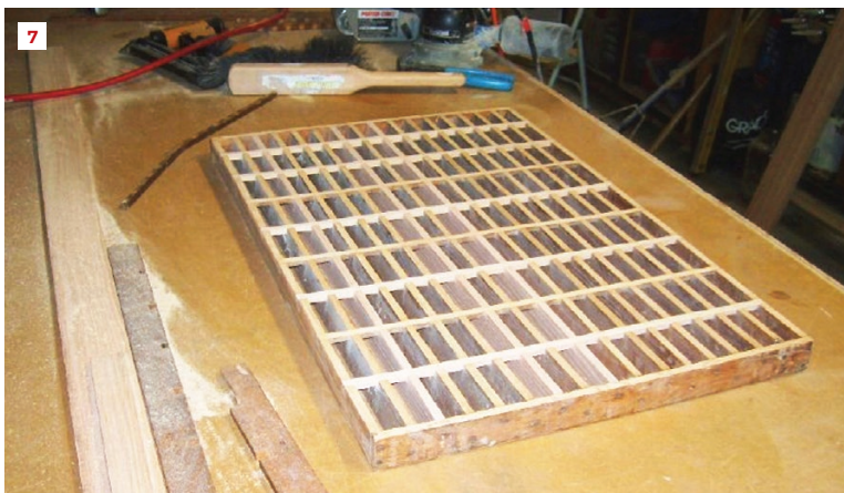
The author uses a table-saw sled (6) with a cleat fixed to the plywood that's the same width as the dado. The cleat is placed at the distance between successive dado cuts (in this case about 4 inches for an adjustable shelf system). He used a similar sled to cut the cross laps for a wooden HVAC floor register (7) and for a Craftsman-style wall screen (8).
