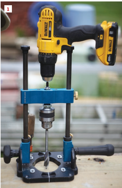
The Rockler portable drill guide has a \frac{1}{2} -inch Jacobs chuck with a \frac{1}{4} -inch hex shank on top that works easily with most drills (1, 2). To accurately drill \frac{5}{8} -inch-diameter holes through a 4x4 post and 2x10 ledger, the author first drilled \frac{1}{4} -inch-diameter pilot holes (3), then switched to a \frac{5}{8} -inch-diameter bit to finish the holes (4).
