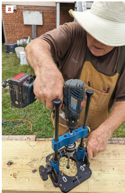
The Rockler portable drill guide has a \frac{1}{2} -inch Jacobs chuck with a \frac{1}{4} -inch hex shank on top that works easily with most drills (1, 2). To accurately drill \frac{5}{8} -inch-diameter holes through a 4x4 post and 2x10 ledger, the author first drilled \frac{1}{4} -inch-diameter pilot holes (3), then switched to a \frac{5}{8} -inch-diameter bit to finish the holes (4).
