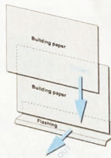
Figure 71. Layer your liquid water control materials to keep the water moving down and out from the house. [Courtesy of Joseph Lstiburek]
