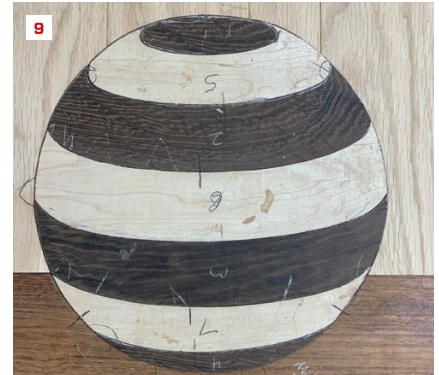
The author makes anchor marks to keep the pieces in alignment as he refines the fit (8). With the various marks the author uses, he is able to highlight points of reference and areas to be removed (9).
