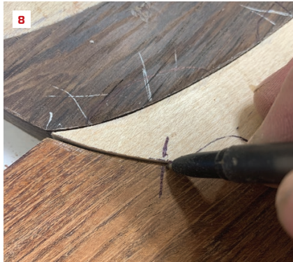
The author makes anchor marks to keep the pieces in alignment as he refines the fit (8). With the various marks the author uses, he is able to highlight points of reference and areas to be removed (9).
