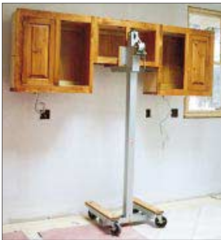
Figure 1. The Gil-Lift allows a person working alone to lift up to 300 pounds of cabinets and maneuver them into place.
