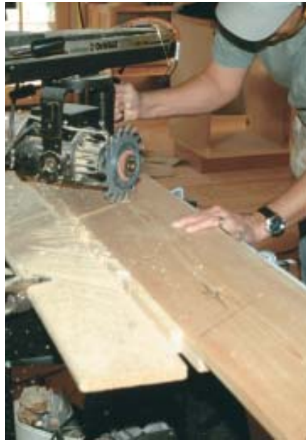
Figure 6. A Forstner drill bit outlines the nosing profile on the housed stringer. The housings are completed with a wobble-dado blade in a radial-arm saw and cleaned up with a straight bit in a hand-held router.
