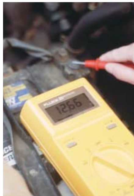
Figure 5. Testing DC voltage, car battery. Reversing polarity causes the needle to fly off the scale in the opposite direction on an analog meter, or read in the negative on a digital unit (left). Reversing the probes will give an accurate measurement (right).
