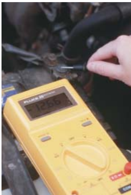
Figure 5. Testing DC voltage, car battery. Reversing polarity causes the needle to fly off the scale in the opposite direction on an analog meter, or read in the negative on a digital unit (left). Reversing the probes will give an accurate measurement (right).
