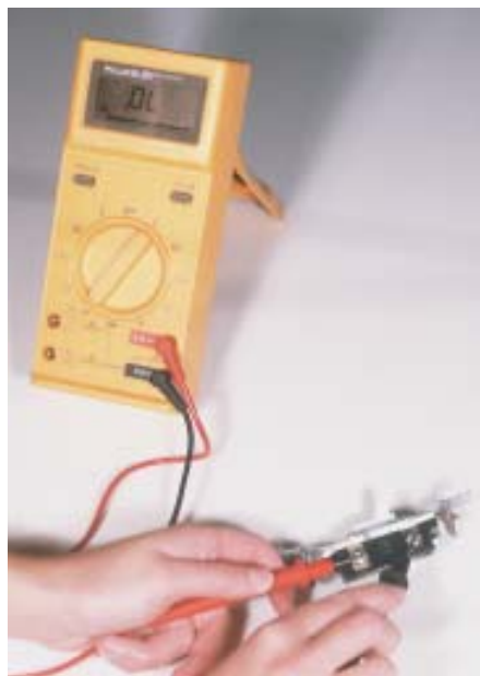
Figure 2. Tone continuity test, switch. With the probes on the terminals and the switch in the off position, there should be no tone. But when the switch is in the on position, a tone should be audible. No tone in either position or a tone in both positions means that the switch is faulty.
