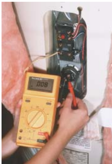
Figure 4. Resistance test, water heater element. A reading of about 13 ohms (4,500 watt/240 element) indicates that this water heater element is functioning correctly.
