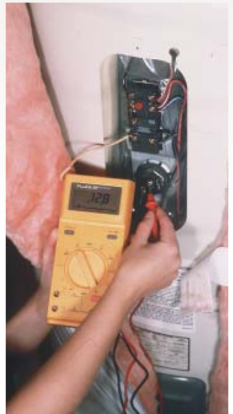
Figure 1. Tone continuity test, water heater element. A properly functioning water heater element should produce a tone in a quality VOM when the probes are touched to the screw terminals. But getting a tone with one probe on the element and the other on the heater body most likely indicates that there's a cracked element shorting to the water. Failing either test means replacing the element.
