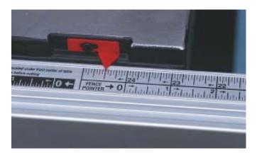
The rear scale on Bosch's saw is especially easy to read because the graduations vary in length and the indicator is right down on the numbers.
