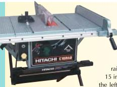
The C10RA2 is an updated version of a saw that came out in the late '90s. Upgrades include a removable folding stand and a cord wrap. The most unusual thing about this machine is the large table, just over 34 inches across. This allows you to make wider rips than are possible with other fixedrail machines. However, the maximum rips of 15 inches to the right of the blade and 16 inches to the left are considerably less than you can rip on a more compact saw with telescoping rails.
