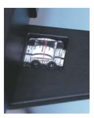
Porter-Cable puts a magnifier over the indicator on its scale. The fence can be recalibrated by loosening the screws and moving the indicator.
