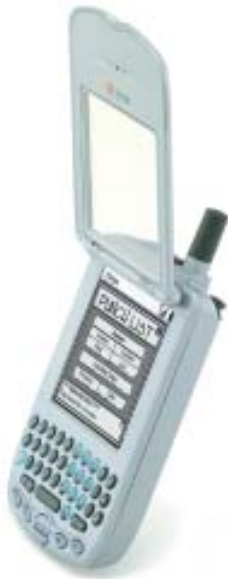
Figure 2. Today, Punch List can run on this Handspring Treo 300, which couples a cell phone with a PDA, complete with thumb keyboard for stylus-challenged users.
