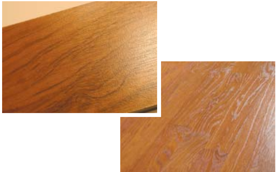
Figure 2. Basic embossing, imprinted in the clear wear layer, imparts a wood texture to the product's surface, but nonaligned patterns that don't follow the wood grain still look fake close up (left). In-register embossing exactly follows the photographic wood grain and achieves a more convincing appearance (right).
