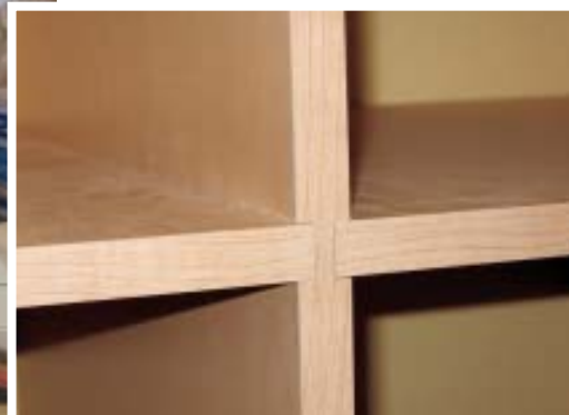
Figure 6. There are a lot of ways to support fixed shelves, but the author prefers dados (left) because they're fast and hide any chipping that occurs when the shelves are cut to length. With the right-size router bit, he can get a tight fit (above).
