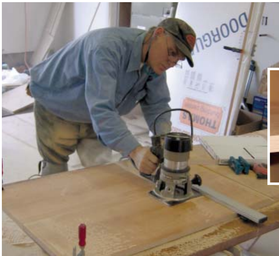
Figure 6. There are a lot of ways to support fixed shelves, but the author prefers dados (left) because they're fast and hide any chipping that occurs when the shelves are cut to length. With the right-size router bit, he can get a tight fit (above).
