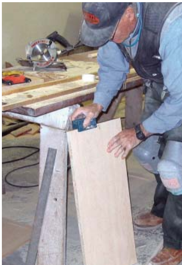
Figure 4. The author uses peel-and-stick vinyl tape to edge areas where the particleboard core is exposed. Here, he uses a dual-blade trimmer to cut the tape flush to the face of a melamine shelf. This trimmer also works on wood veneer edging.
