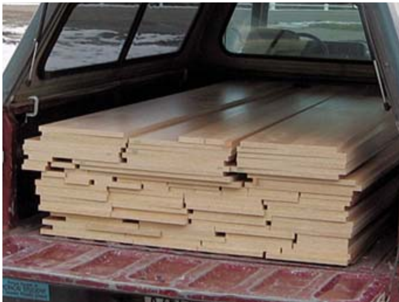
Figure 1. The author buys the entire closet package from a cabinetmaker who rips melamine into shelves and cleats before banding them with a matching edge (above). This nearly eliminates ripping and edging material in the field and allows customers to get highly customized shelving in virtually any color or pattern they want.
