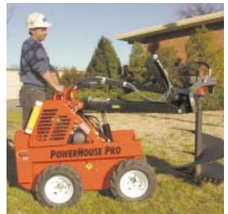
Although the PowerHouse Pro's rubber tires are gentle on grass, its short and narrow wheelbase makes it tippy and potentially dangerous on uneven or hilly terrain.
