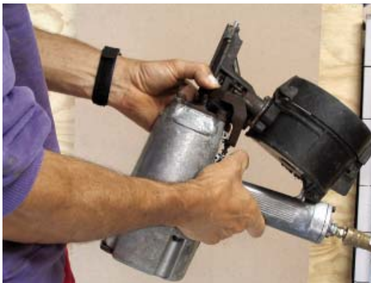
Figure 4. To check a nailer's driver without disassembling the tool, dry-fire it (with fasteners removed) while keeping the trigger depressed.
