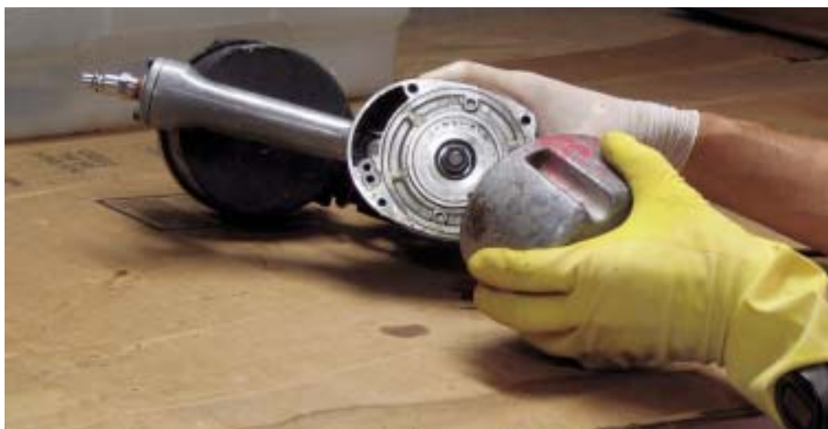
Figure 5. After carefully removing the cap screws (left), the author takes off the cap to expose the cylinder and piston inside (below). Working on a large piece of clean cardboard makes it easy to keep track of parts and to clean up afterward.
