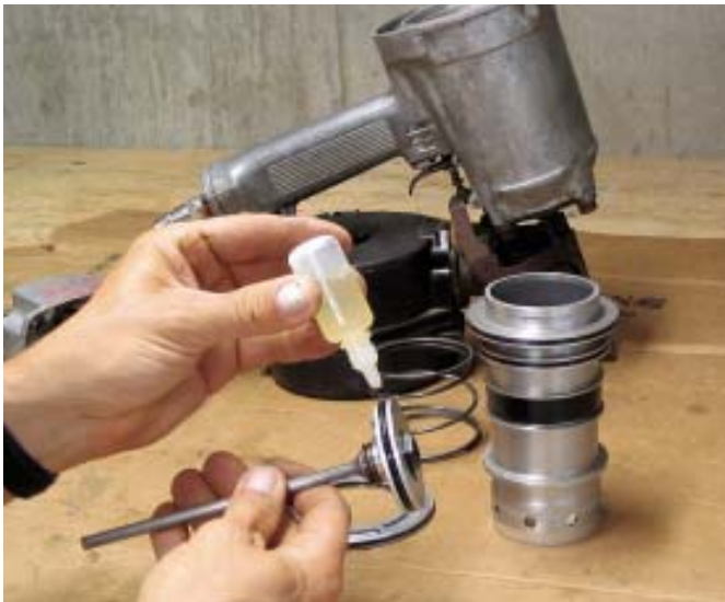
Figure 9. Before inserting the piston into the cylinder, the author spreads a thin coat of lubricant on the interior of the cylinder and on the piston's new O-ring (left). After aligning the driver with its slot inside the piston (right), he eases the piston back into the cylinder, taking care not to damage the O-ring.
