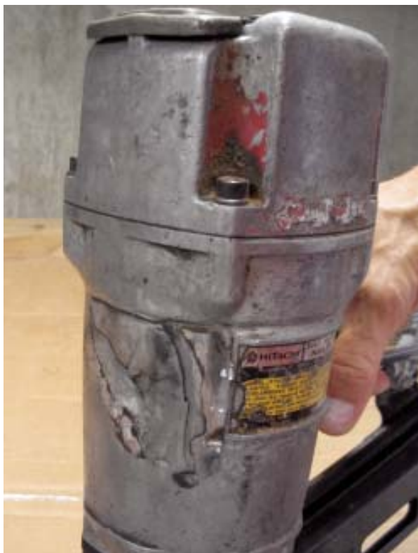
Figure 3. An air tool with a cracked body is potentially dangerous because it can blow apart. It should be removed from service.
