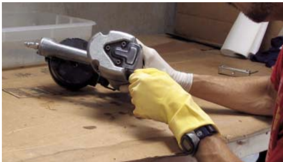
Figure 5. After carefully removing the cap screws (left), the author takes off the cap to expose the cylinder and piston inside (below). Working on a large piece of clean cardboard makes it easy to keep track of parts and to clean up afterward.
