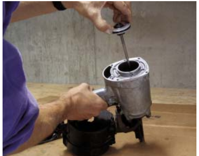
Figure 9. Before inserting the piston into the cylinder, the author spreads a thin coat of lubricant on the interior of the cylinder and on the piston's new O-ring (left). After aligning the driver with its slot inside the piston (right), he eases the piston back into the cylinder, taking care not to damage the O-ring.
