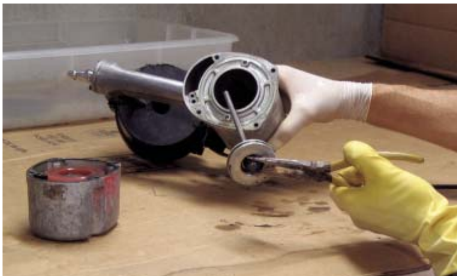
Figure 6. Some pistons have a nut on the top that can be grasped with a pair of needle-nose pliers, making it easier to pull the piston out of the cylinder.
