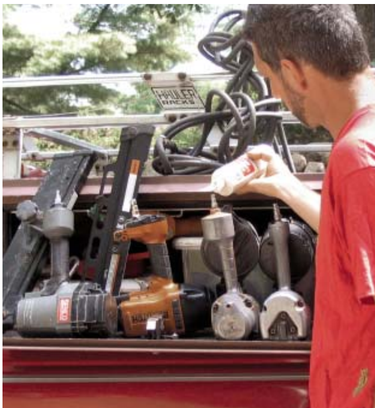
Figure 2. Nailers should be oiled on a daily basis with lubricants designed specifically for pneumatic tools.
