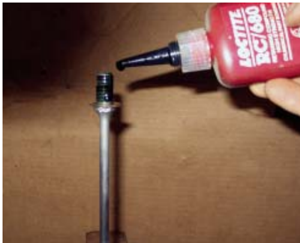
Figure 8. The author uses a thread-locking compound when reassembling a piston and its threaded or bolt-on driver.
