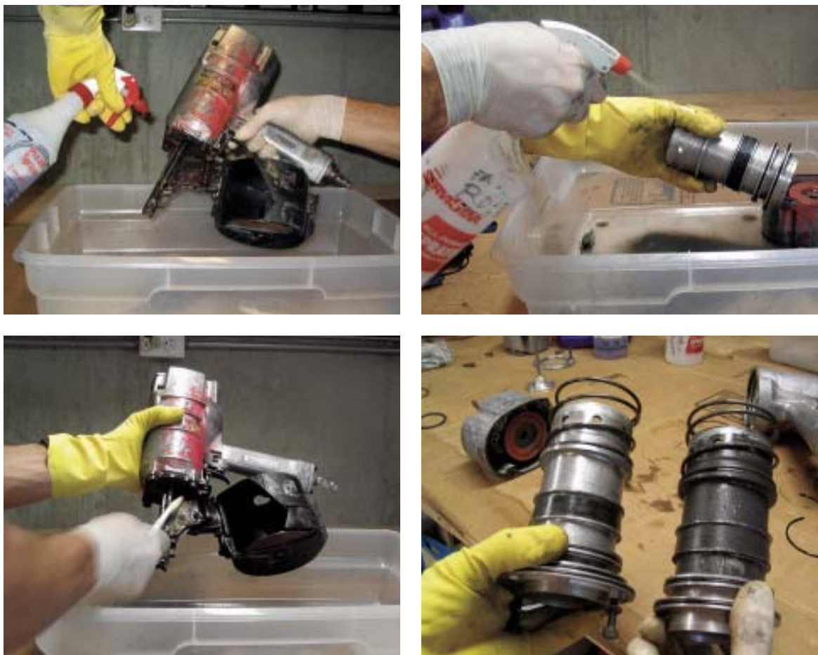
Figure 7. A biodegradable automotive degreaser is an effective cleaner, and can be sprayed on both the exterior and interior of the tool (top left). Most tools can simply be rinsed with water afterward (top right). A toothbrush is perfect for removing stubborn dirt (above left). Two cylinders — one clean and one dirty — demonstrate the importance of regular cleaning (above right).
