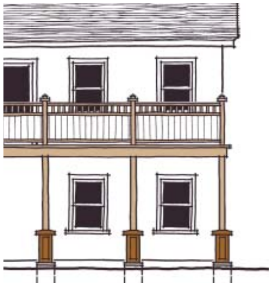
Boxed-in deck posts appear to be standing on raised piers
