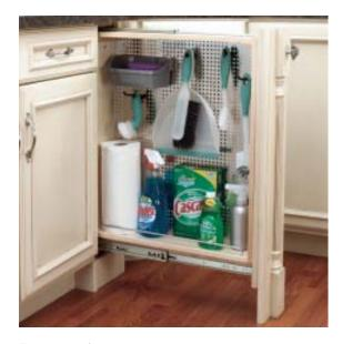
Pegged. The perforated stainless-steel panel in Rev-A-Shelf's new *kitchen-cabinet* organizer allows everything from pots and utensils to cleaning implements to be hung on hooks. The 6-inch rollout shown — one of several models available — includes three full-extension ball-bearing slides and fits cavities 30 inches high and 23 inches deep. It costs about \$175.
