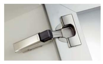
Slamproofing. Blumotion is an integral braking system that brings swinging cabinet doors gently to rest. It comes in several models and can be added to cabinets after they're installed. The model shown simply clips onto the arm of a Eurostyle hinge. It costs about \$6.
