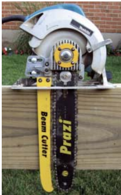
Figure 5. For 6x6 or 8x8 posts or for large beams, this chain-saw attachment for a circular saw will do the job faster and cleaner than a reciprocating saw can. Without the attachment, cutting through thick material would take several passes with a circular saw.
