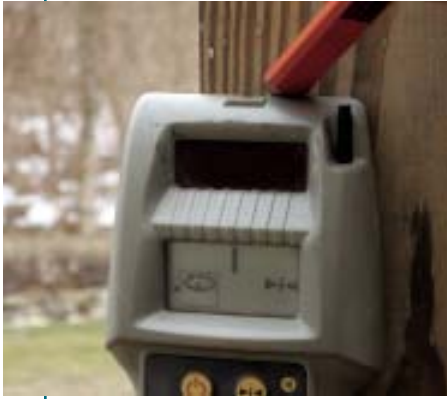
Figure 2. The electronic hand-held receiver for a laser level has an infrared sensor that locates the level line precisely, which gives the builder an accurate reading for making cutoffs after over-sized posts have been placed and plumbed into position.
