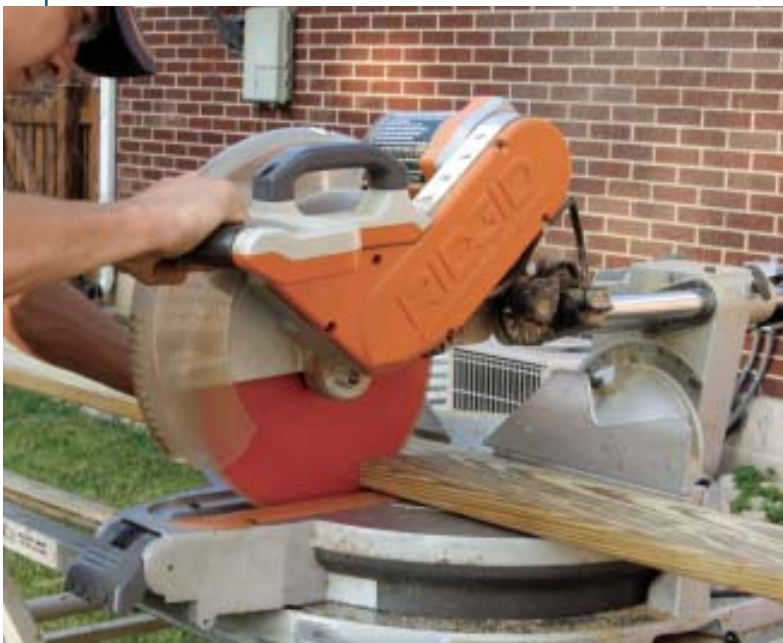
Figure 9. Time spent can also be time saved. The improved accuracy and the quality of the cut afforded by using a miter-saw instead of a circular saw can outweigh the additional time it takes to bring the workpiece to the tool.
