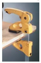
third hand. The cam-actuated *Quick-Jaw PowerCam Clamp* works one-handed and can provide over 500 pounds of clamping pressure. The signature "power cam" uses a ratcheting lever, providing greater force with more precision than screw-adjusted clamps. Large non-marring pads feature an integral V-groove to allow clamping of pipe or dowels, and a quick-release button on the
