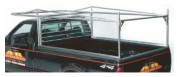
steel. They feature heavy-duty welded construction and capacities from 700 to 1,000 pounds (depending on the model). Most include adjustable ladder positioners. The starting price for pickups with a cap is \$600; for pickups without a cap, they start at \$550; van racks start at \$290.
