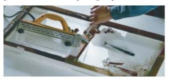
vaporize lead, and the scraping technique reduces the amount of toxic, airborne particles produced by grinding or sanding. The tool sells for \$395 and includes a handsfree attachment for use on vertical surfaces.
