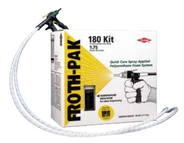
Foam Pack. Typical fiberglass insulation is virtually useless for insulating band joists and other leaky areas. A much better option for these problem spots is a two-part foam like Dow's Froth-Pak 180. The kit — which includes an applicator gun with an 8-foot hose — yields about 18 board feet of insulation; other sizes are available for bigger and smaller jobs. I found the Froth-Pak 180 online for about \$300.
