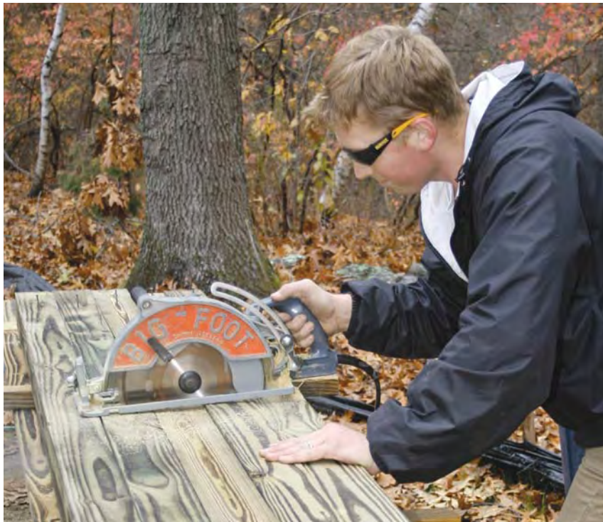
Figure 8. The right tool can be a big timesaver: The Big Foot Saw Adapter allows for a 10 \frac{1}{4} -inch blade in a standard Skilsaw and cuts 4-inch stock in one pass.
