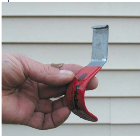
Figure 14. A J-shaped zip-lock tool (above) grabs the bottom lip of vinyl siding, disengaging it from the course below (right).
