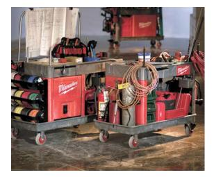
On the Move. There are lots of ways to move tools around a job site — in a shopping or food-service cart, on a dolly, even in a little red wagon — but Milwaukee's *Trade Titan* is actually made for the job. Waist-high, it provides a stable work surface on durable casters capable of supporting 450 pounds apiece. It comes in two models: the 48-60-5010, with an open bottom (\$344); and the 48-60-5015, with a cabinet bottom (\$430).
